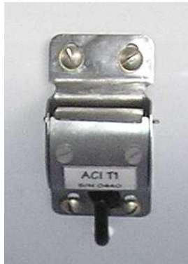
Fig.1- Stall speed vane on the left wing
